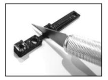
1. Using a sharp modeling knife or cutters, separate the two adaptors from the sprue.
